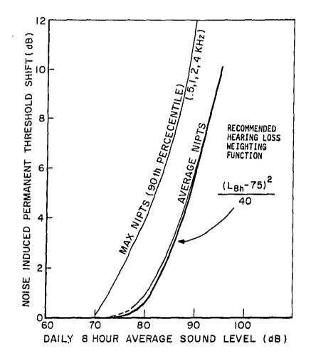
Figure VI-2. Potential hearing damage risk for daily exposure to 8 hour average sound levels. The curves predicts noise induced permanent threshold shift (NIPTS) in octave bands (.5, 1, 2, 4 kHz) for 8-hour exposure at various continuous noise levels. The eight hour average sound level can be replaced by DNL with negligible error if a person spends the remaining 16 hours out of 24 in L of 70 dB or lower.
